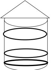
Why are the hoops closer together near the bottom of the water tower?
